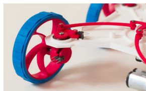
An electromechanical system with combination of parts made in AM and non AM processes
