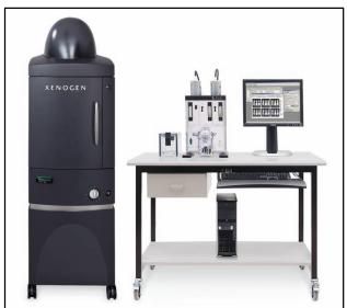
**Figure 1. Proposed Imaging Equipment for New Imaging Core.** The IVIS Spectrum system from Caliper Life Sciences enables 3D live-animal optical imaging. Images generated from here will then be further processed by UH's cadre of computational image analysis researchers.
